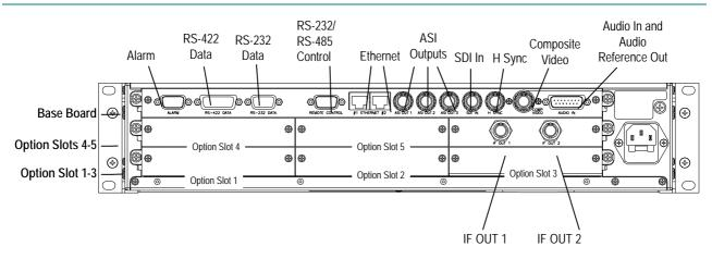
Figure 2.7: E5750 (2U) Rear Panel Component Parts and Connectors
